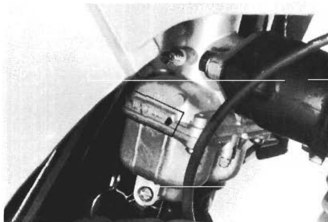
The carburetor identification number is on right side of the carburetor body.
