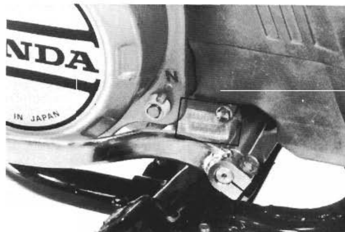
The engine serial number is stamped on the lower left side of crankcase.
